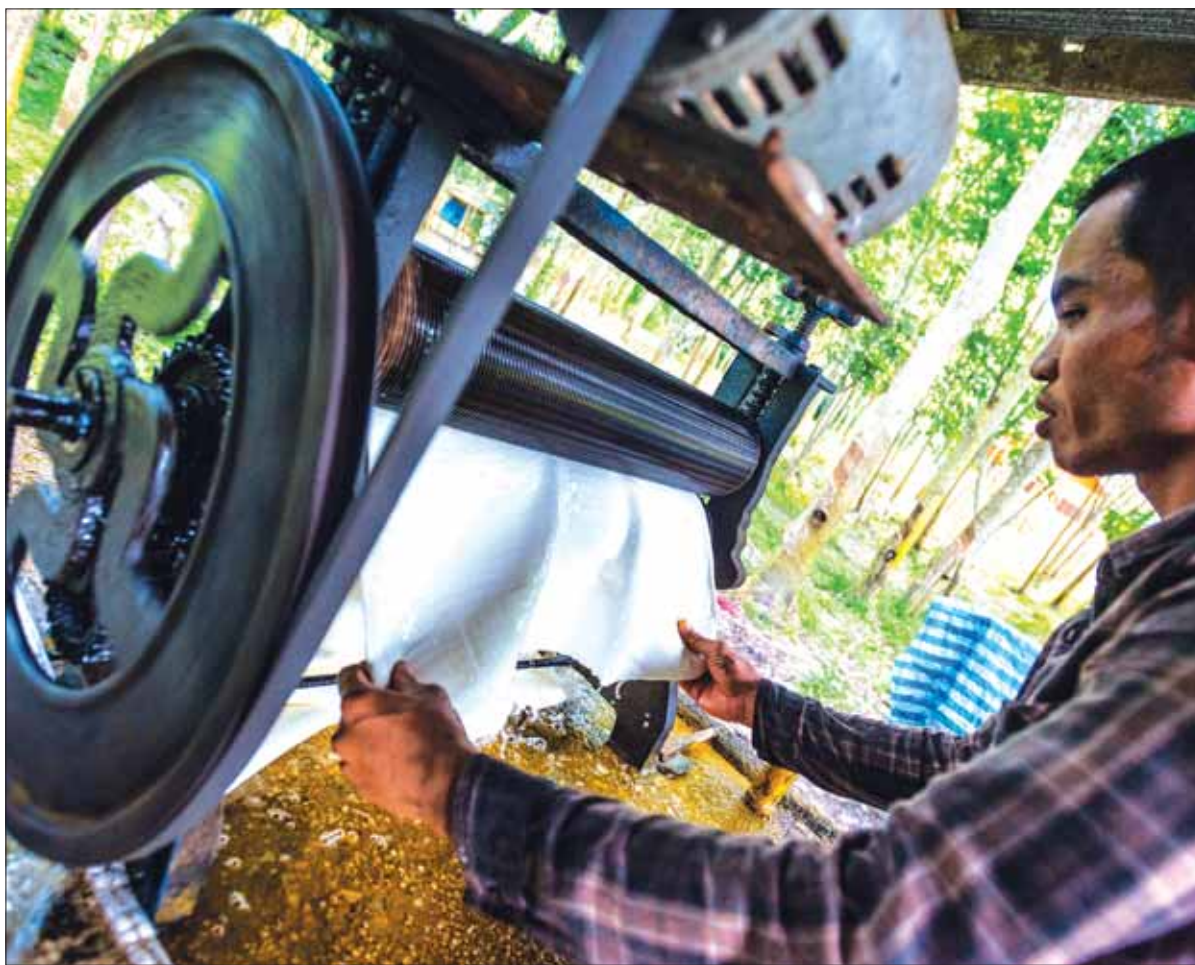
A plantation worker feeds fresh rubber sheets through a series of rollers to remove moisture. Photo: Jeremie Schatz
