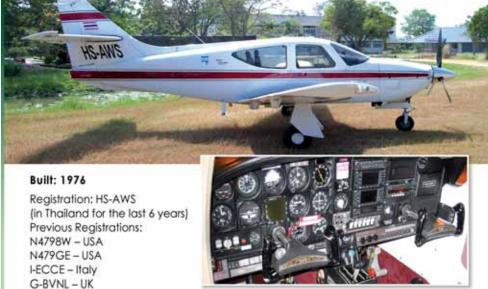
Lycoming IO-540-T4B5D (1,300 hours, 700 hours to TBO). Prop: B3D32C419/82NHA-5. Overhauled Feb 2011 (7 years to TBO). C of A Due 11th November 2011. New 5-year Permit. 100 hour check completed 19 Feb 2011.
