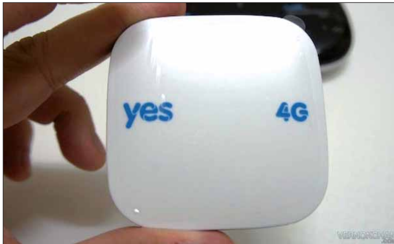
HERE, THERE, ANYWHERE: Yes’s 4G Huddle XS. It’s a 4G MiFi device that can provide internet or network access to any WiFi enabled peripheral device at a distance up to 10 meters (30 feet). Photo: Vernon Chan
