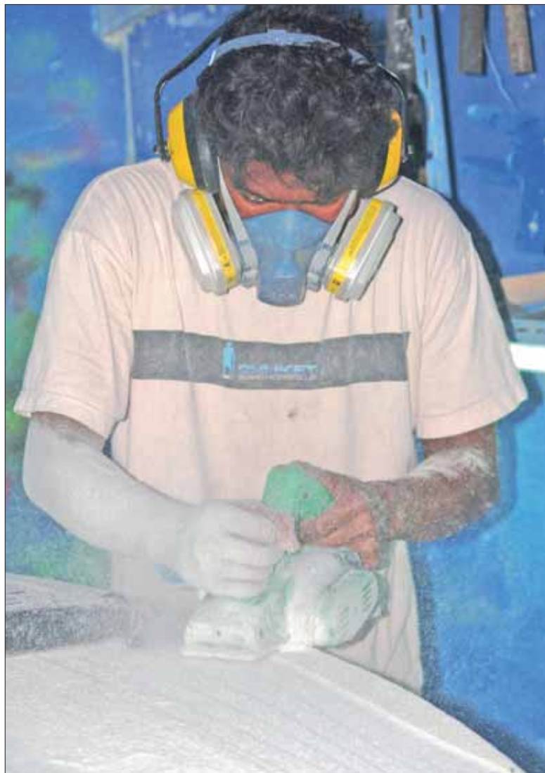
SANDMAN: Using an electric sander, Tony shapes a board blank inside a sealed room that is significantly hotter than outside.
