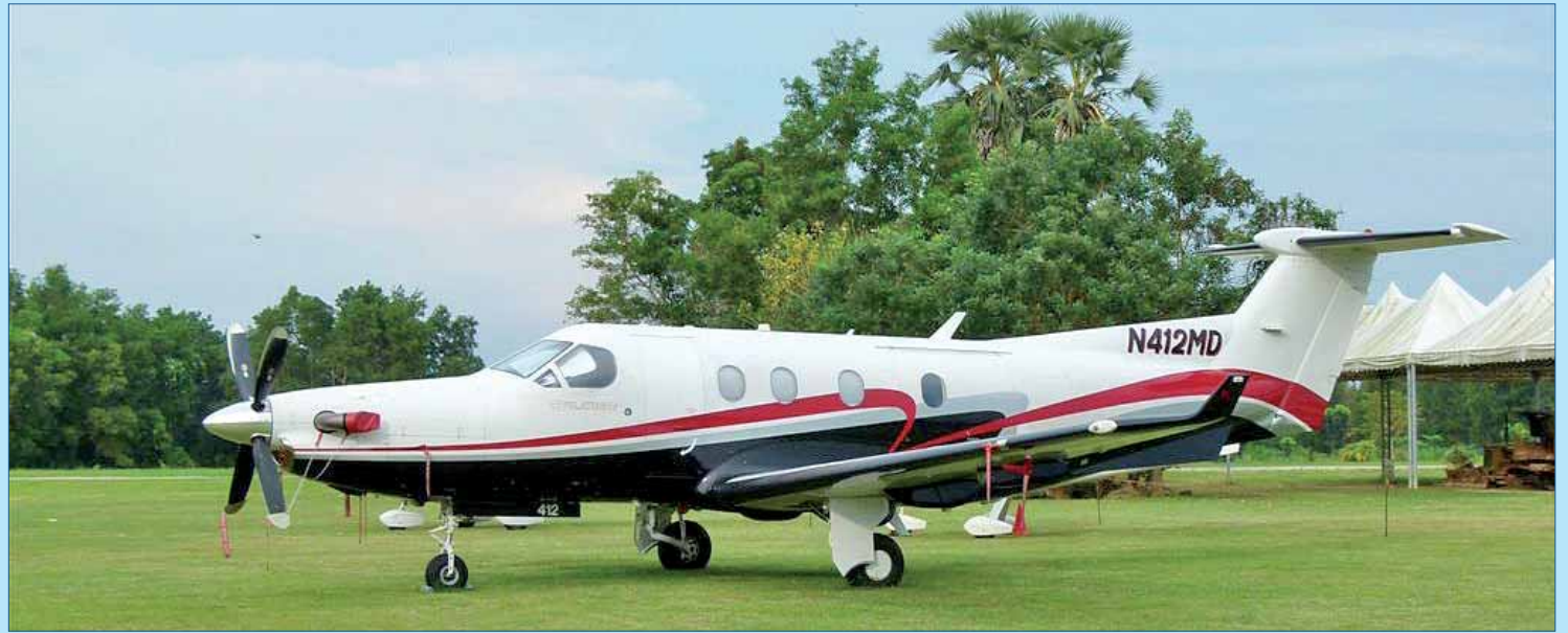
IT'S PLANELY BEAUTIFUL TO SEE: The Pilatus PC-12 is powered by a single Pratt & Whitney Canada PT6 turboprop engine.
