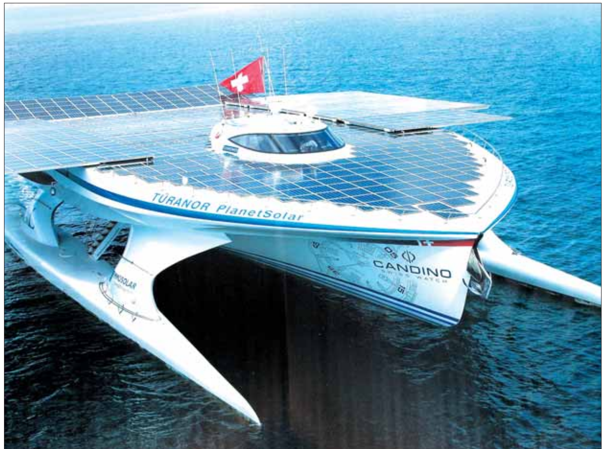
HERE COMES THE SUN: The MS Turanor PlanetSolar 's multihull is topped by a massive array of photo-voltaic solar panels that at full exposure cover an area of 537 square meters. Photos by Warisa Temram
