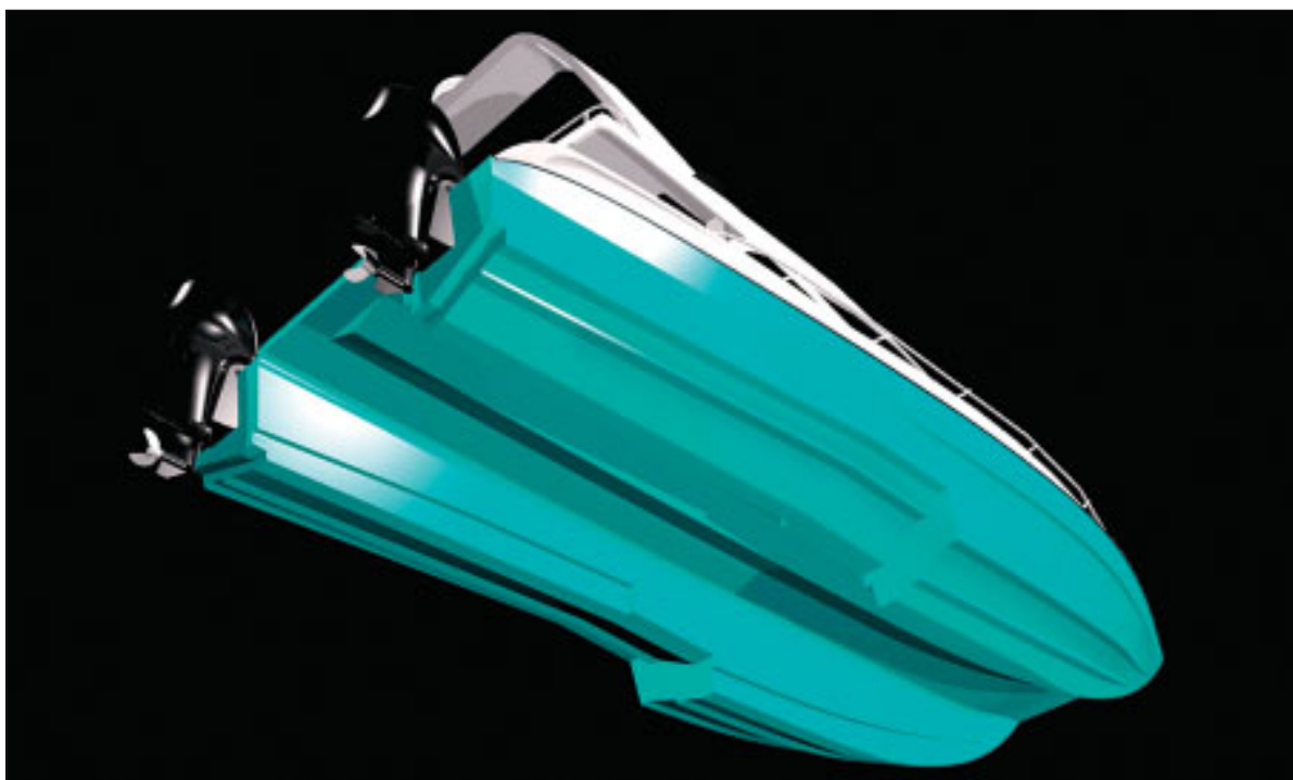
A fish's-eye view of a stepped-hull catamaran. The step creates a cushion of air, reducing drag.
